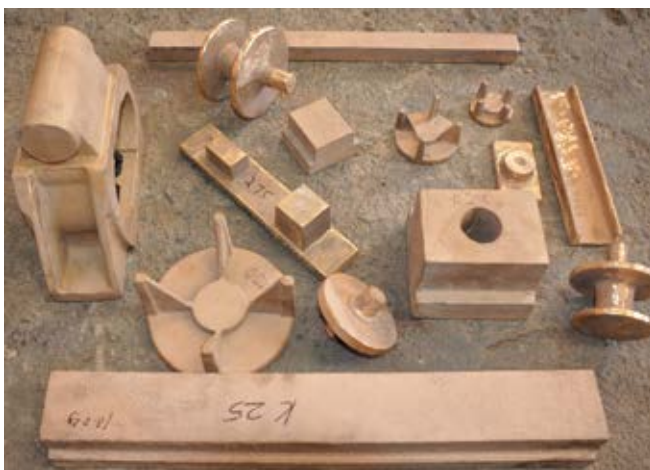
Various components that Intervention Engineering has cast. The company has cast kick plates, stoppers, beam guides, side walls and channels mainly for the mining, power and general engineering industries
